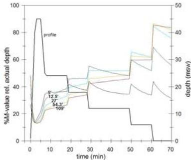
Fig. 1 Calculated %M-values (left axis) of standard simulation (depth on right axis). Numbers are  $t_{1/2}$ 's. %M-values are < 100% with the liberal ZH-L16C (shown). RGBM DCs have 0 msw deco-c ceilings, but ZH-L8ADT DCs at 3 msw.
