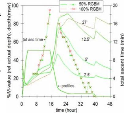
Fig. 6 RGBM-DC with full (100%) and half (50%) "implementation" of RGBM. Left %M-values of ZH-L16C and depth, right total ascent time. After 19 min dive time, 50 and 100% settings yielded identical ascent profiles (as prescribed by DC) and same "total ascent time" displays. NFT 16h22 and 16h15. The smoothed %M-value curves during the "exponential" ascent (<10 msw; compare with Fig. 1) will diminish bubble occurrence.
