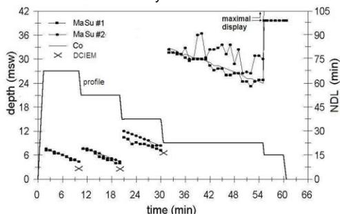
Fig. 3 Large differences of NDLs mainly due to large differences in M-values, not to 1/2 times.
